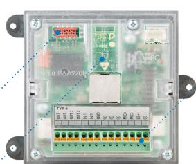
Spring clamp terminals for electrical connection without tools.
