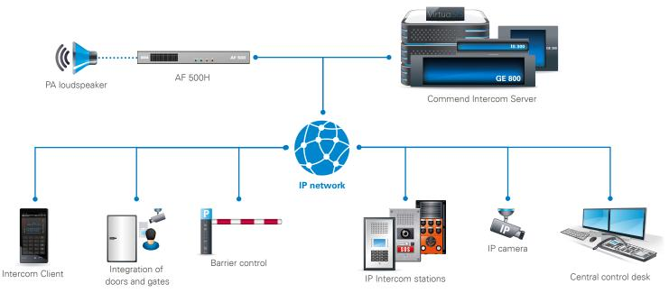
The following illustration shows an example of the integration of an AF 500H amplifier into an IP network.
