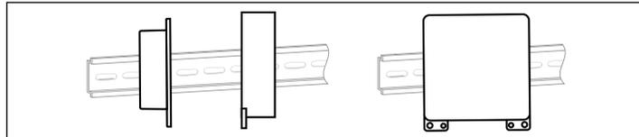
Mounting options with an IP-Bridge: vertical flat and horizontal flat.
